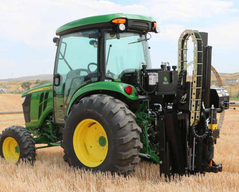
The 9110 Ag-Probe TR is the newest model in the AMS PowerProbe line up. It is designed for use in agricultural and environmental sampling. This model can be mounted on most standard tractors that meet the standard weight limits. The 9110 Ag-Probe TR is powered by the Power Take Off (PTO) from the tractor.
