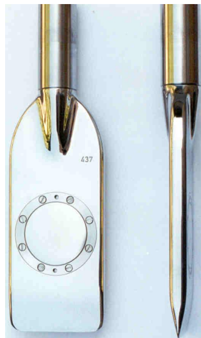
Fig. 1. The flat dilatometer - Front and side view
