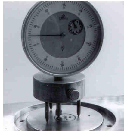
Fig. 14. "Tripod" dial gage
