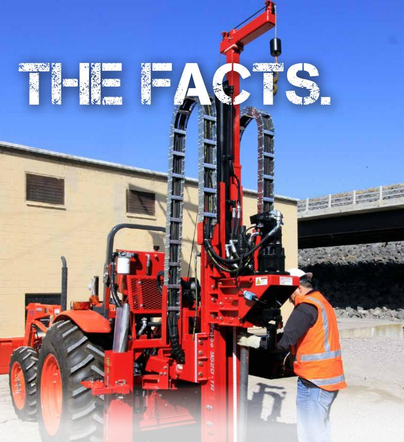
The 9520-TR PowerProbe™ is ideal for remote access when traveling off road for long distances. This comes standard with our 350 ft/lb direct-push percussion hammer. For those situations where you need to install groundwater monitoring wells, you can add our 3,400 ft/lb 2-speed auger drive head and in addition to the auger you can also include the convenience of our 3,000 ft/lb overhead winch line for tripping center rods to speed up sampling in the field.
